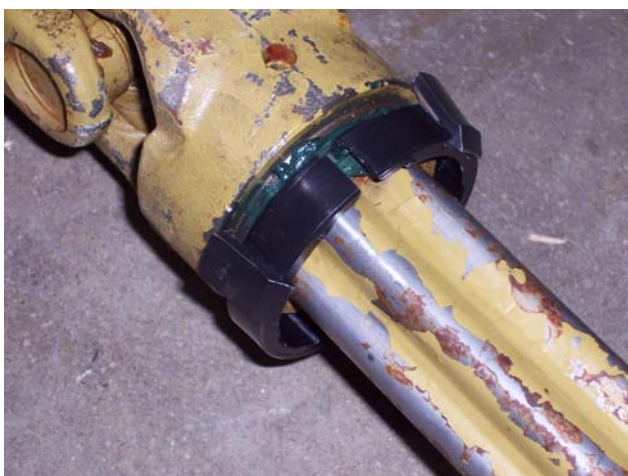
Figure 2. The Nylon Bearing Rides in the PTO Yoke Groove; Lubrication is Recommended.
